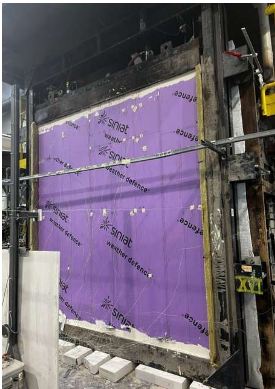
Illustration 1 : Essai 24889A-rev1 REI 60 iQ3 Warringtonfire Gand
